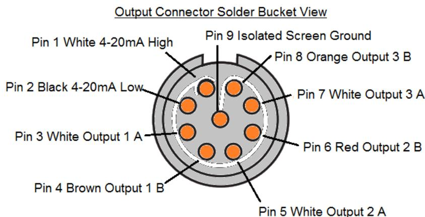
**Figure 15 Output Wiring**
