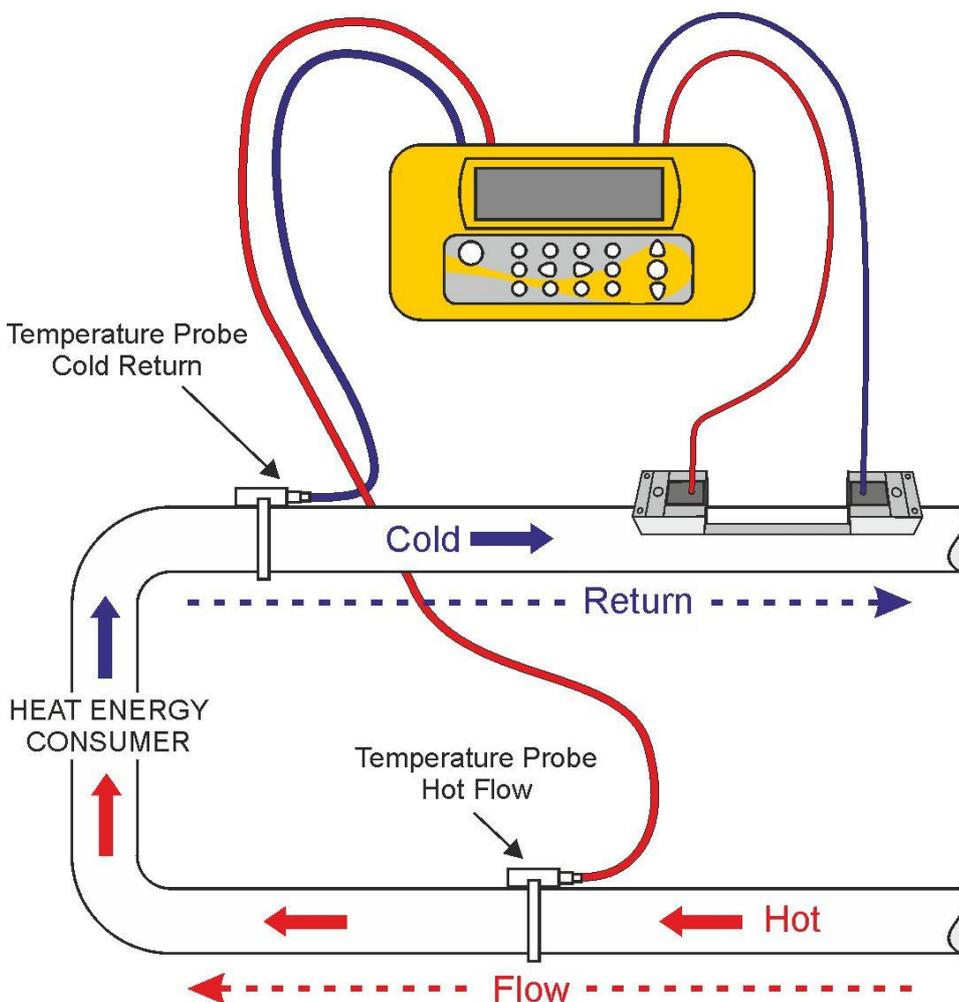
**Figure 13 Portaflow 333 Temperature Probe Positioning (Heater system)**
