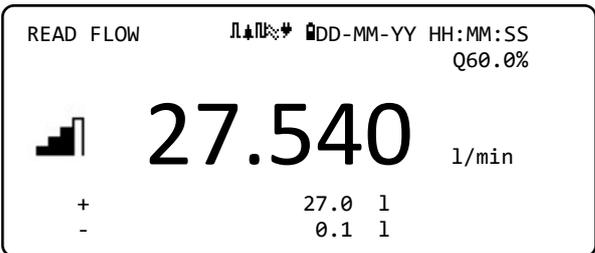
The *Read Flow* screen is used most frequently during normal monitoring operation. It shows the instantaneous fluid flow together with totalised values (when enabled).
