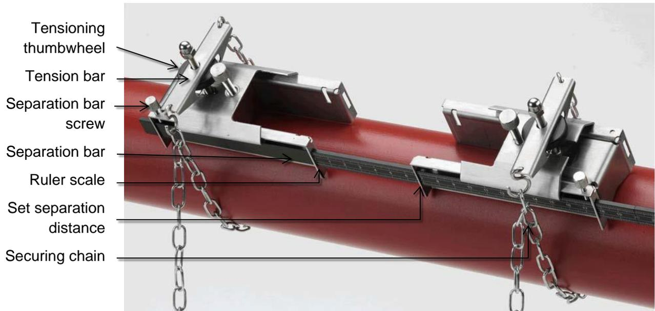
**Figure 9 Guide rail assembly (Reflex Mode)**
