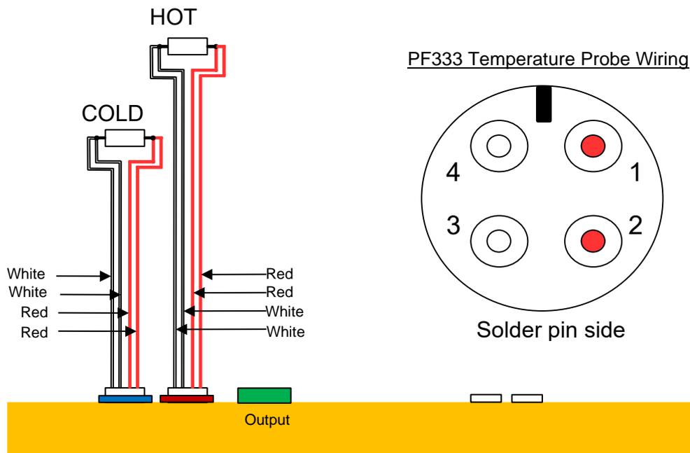
**Figure 14 PF333 Temperature Probe Wiring**
