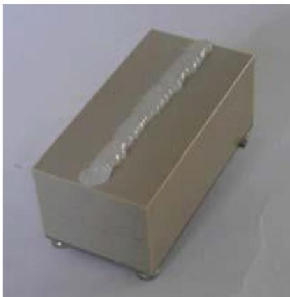
**Figure 10 Applying ultrasonic couplant**
