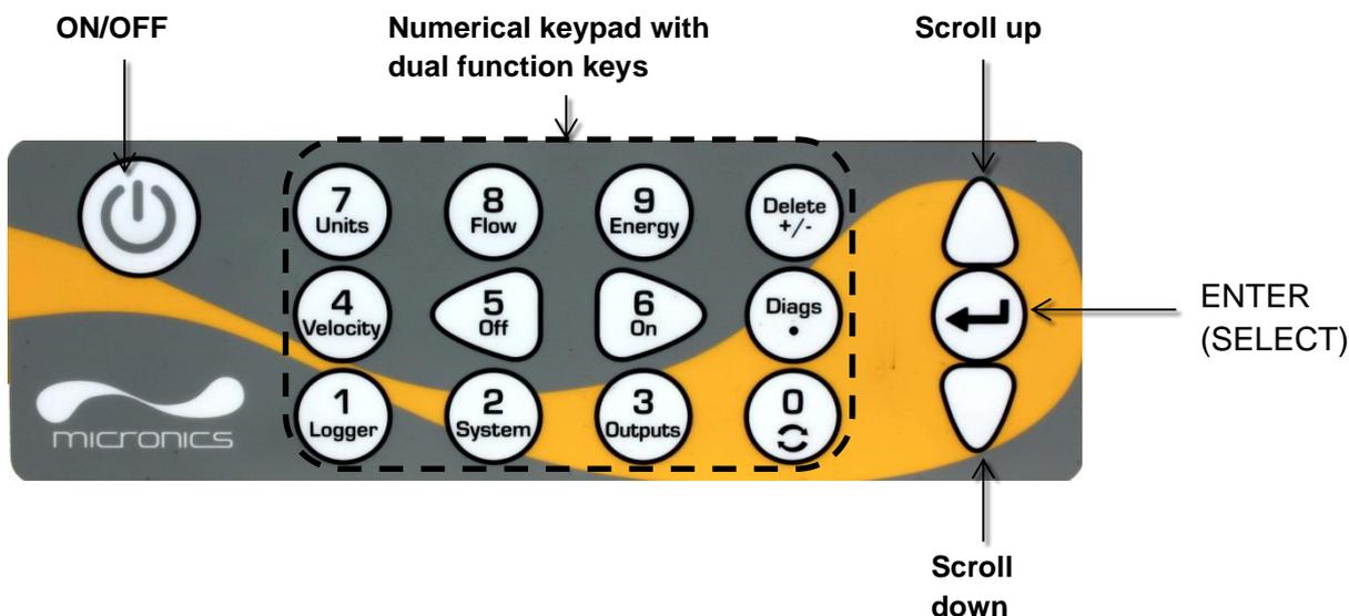
**Figure 6** Portaflow keypad
